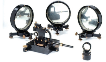
Foucault device for measuring the speed of light, 1865.
